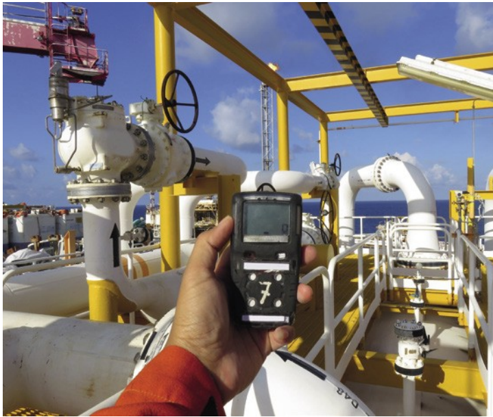
Picture 2: Gas detector: Fugitive emissions of H 2 are imperceptible for human beings
